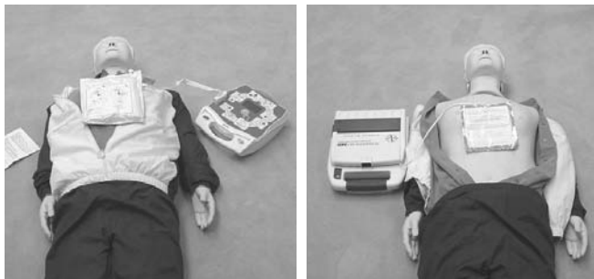
Figure 2. Electrode pads never removed from packaging during use of Zoll (left) and Cardiac Science (right) AEDs.
